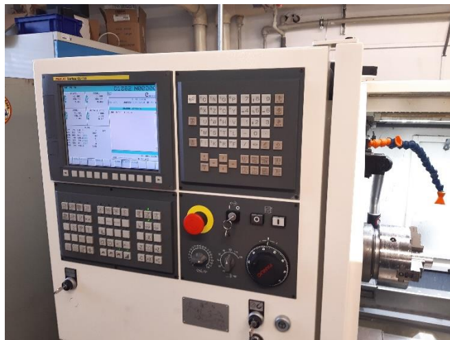
Fig. 35 Control panel (FANUC system).
