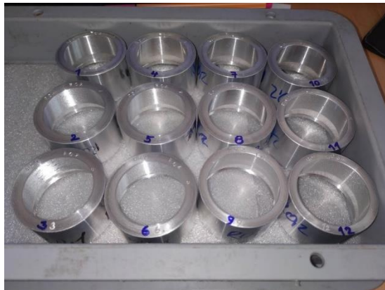
Fig. 37 The samples which were machined under different cutting conditions.
