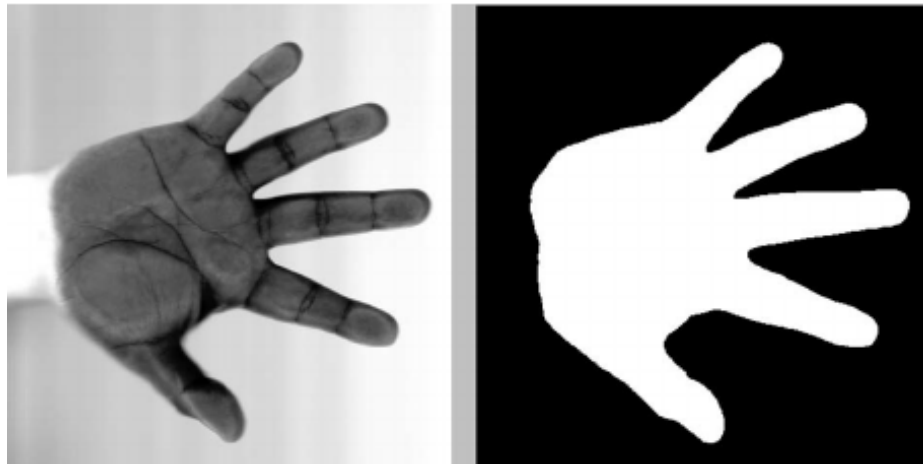
Figure 7: Two-class segmentation on a grayscale picture. Darker parts are chosen as the object, lighter parts are chosen as the background. [25]
