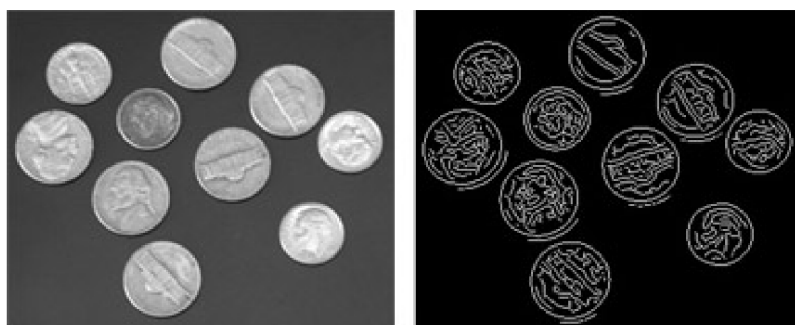
Figure 9: An example of the edge-based segmentation (used on an image of coins). [26]
