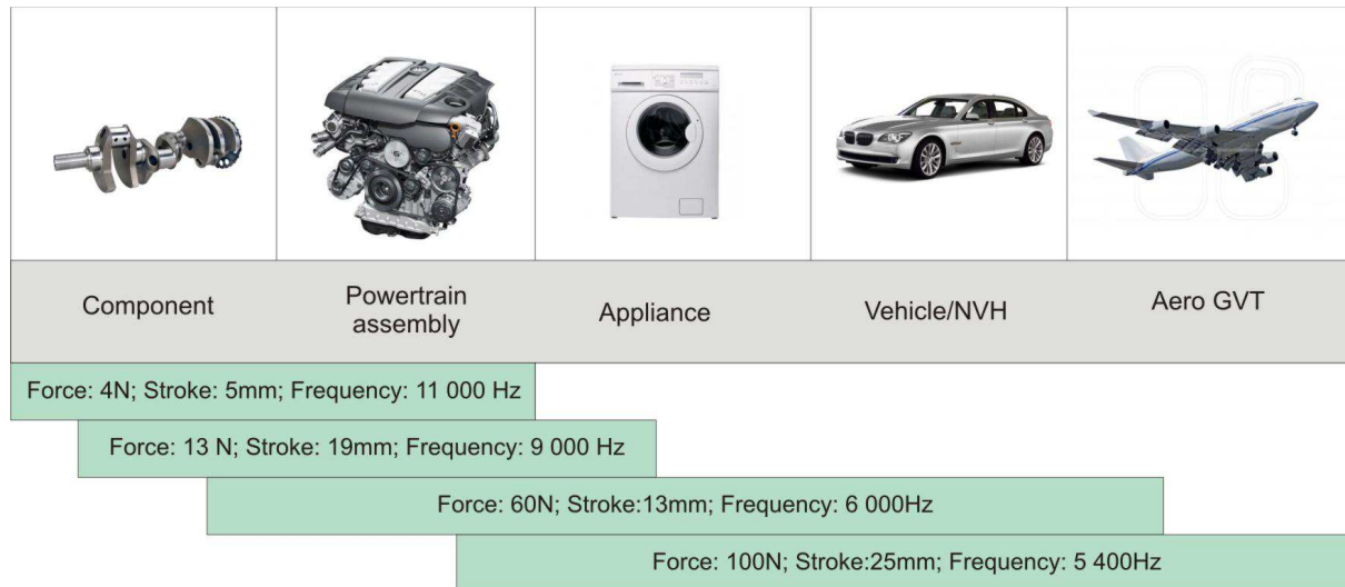
Figure 22 Exciter parameters according to application [19]
