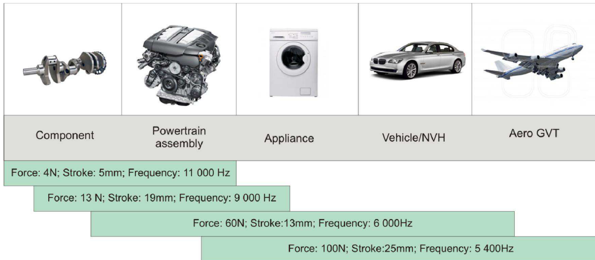
Figure 22 Exciter parameters according to application [19]
