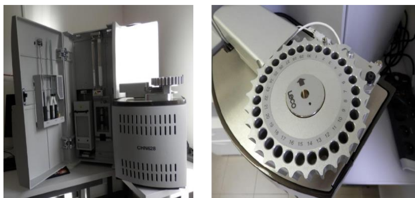
Figure 17. Laboratory equipment LECO CNH628
