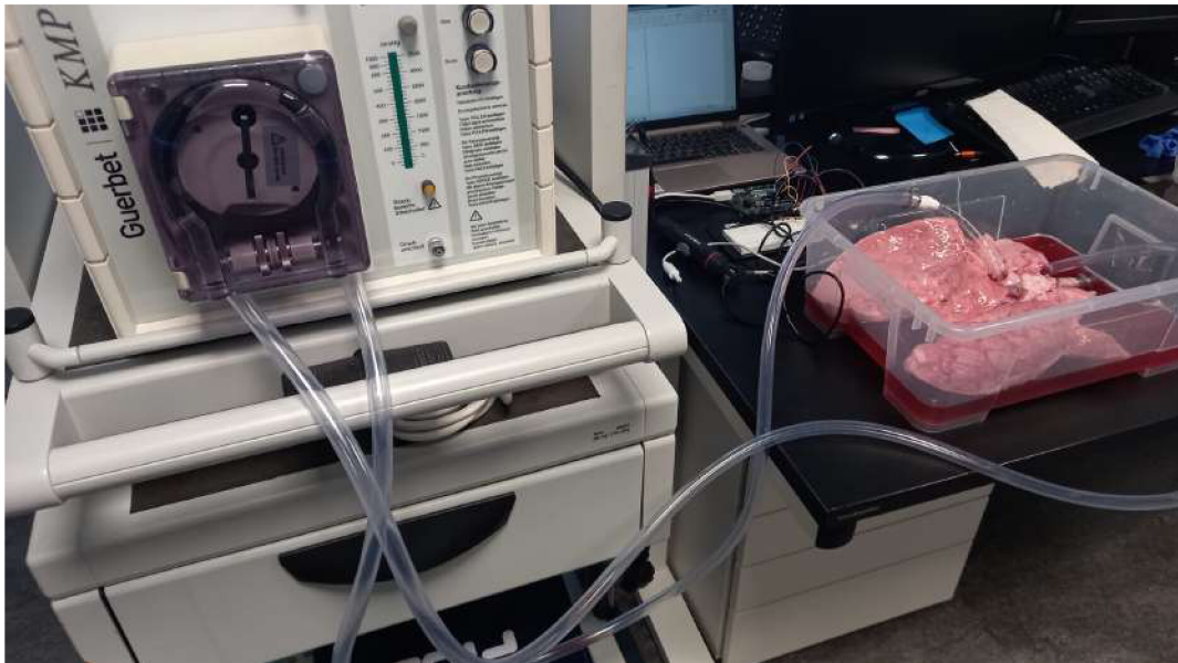
Fig. 2.5: Lungs perfused by using peristaltic pump
