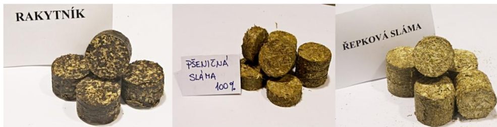
Figure 9.: Briquettes made from pure materials SBT wood chips (left), wheat straw (middle), rape straw (right)
