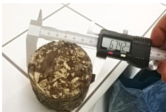
Figure 15.: Measuring the diameter of SBT briquette by Vernier calliper
