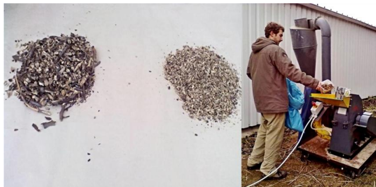
Figure 6.: Wood chips and crushed wood chips (left) and grinding of the wood chips on hammer mill type 9FQ - 40C (right)
