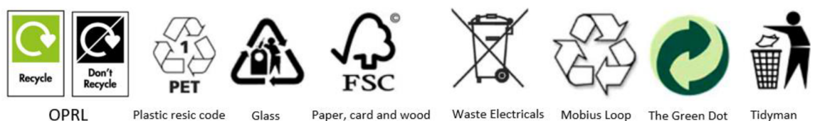
Figure 2 Examples of the most known recycle labels (The Waste and Resources Action Programme (Wrap), 2004)
