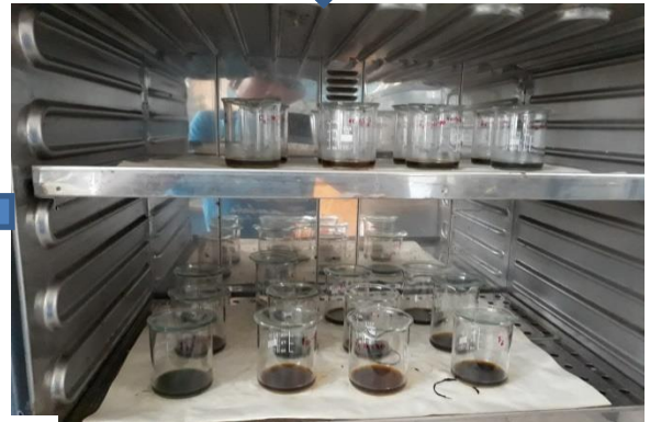
C. Heated soil suspension
