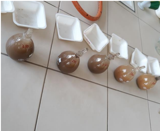
C. Soil suspension in pycnometer
