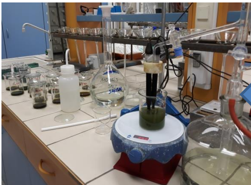
D. Titration with Mohr salt ( (NH_4)_2Fe(SO_4)_2 )
