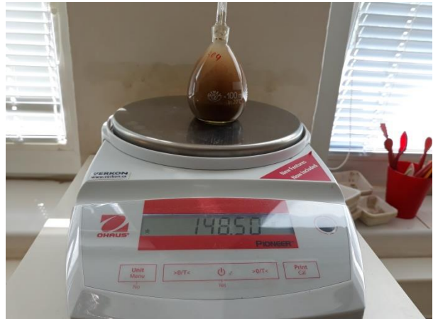
D. Weighted soil suspension
