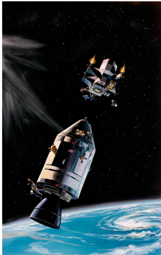
Fig.5. Illustration of docking maneuver of the ascent stage with the Command and Service Modules (NASA, 1969)
