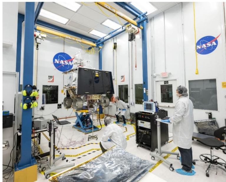
Fig. 11. Testing of VIPER rover's wheel movement and rotation (NASA, 2024)
