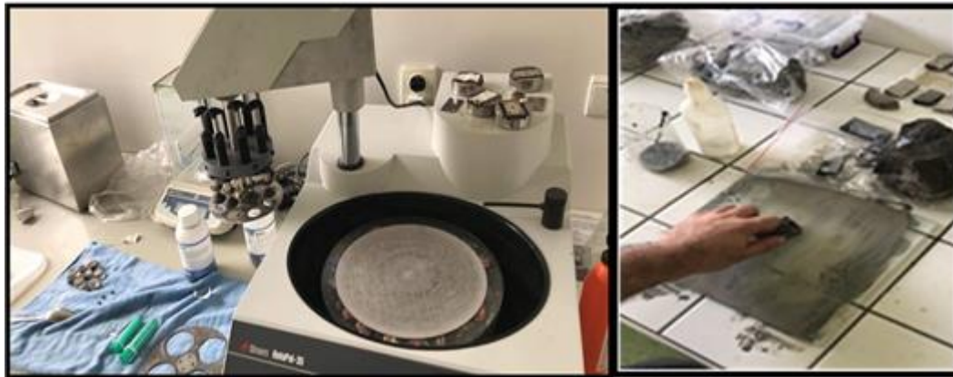
Figure 6: Polishing every samples for thin-section
