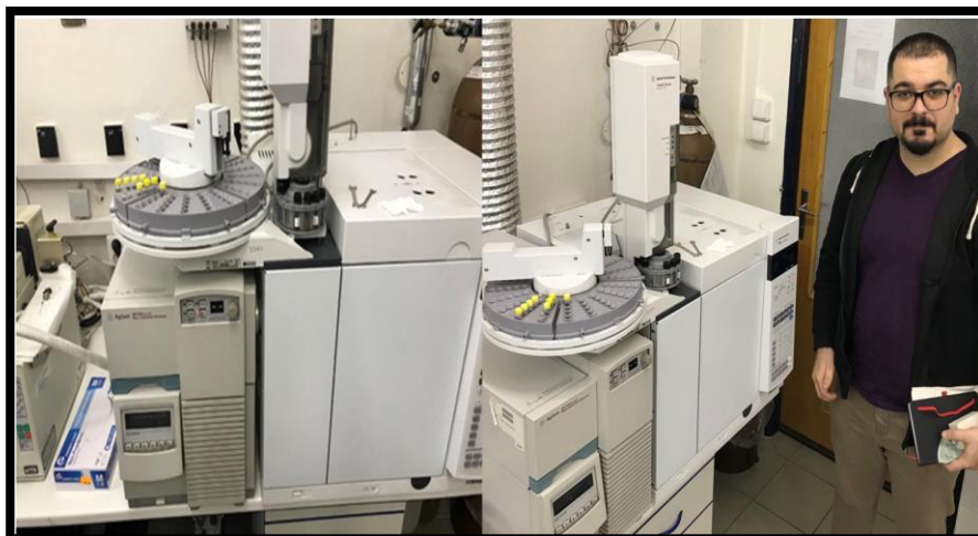
Figure 15: Agilent A6890N chromatograph equipped with Agilent 5973 NMSD quadrupole mass spectrometer (GC-MS)
