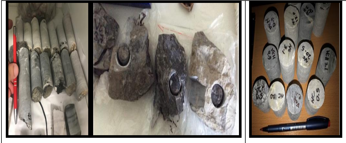
Figure 4: Preparing Core-Plugs from the rock samples
