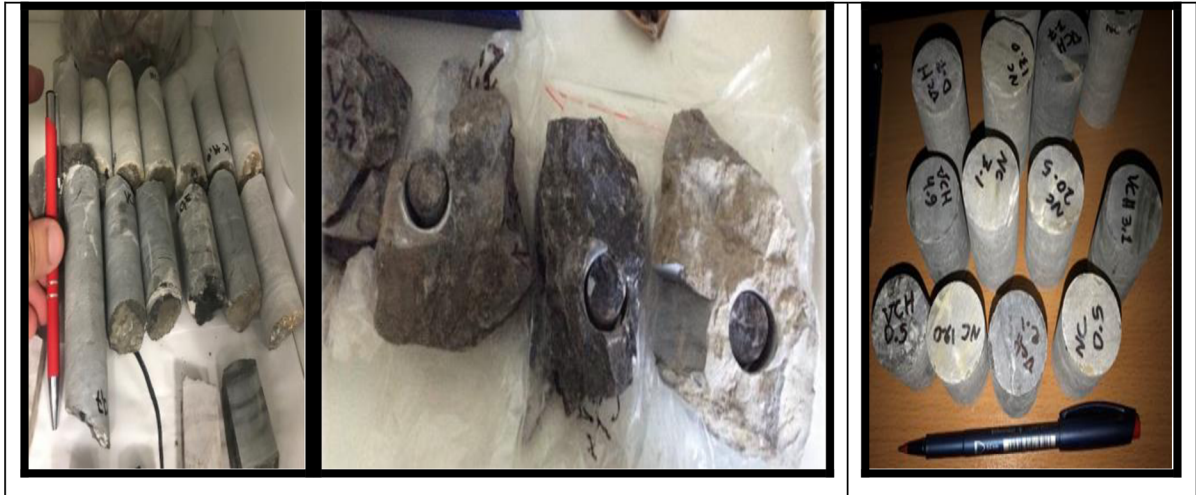
Figure 4: Preparing Core-Plugs from the rock samples
