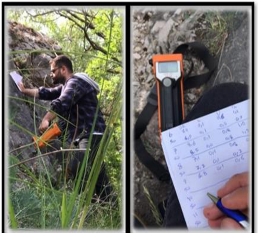
Figure 2: Using the gamma-ray spectrometer equipment at the Field
