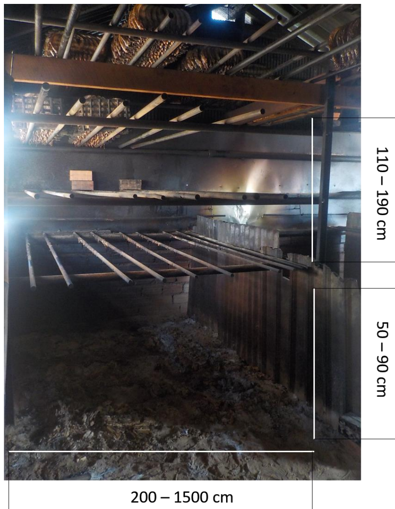
Figure 40 Example of typical smoking kiln dimensions, Tonle Sap area, Cambodia.
