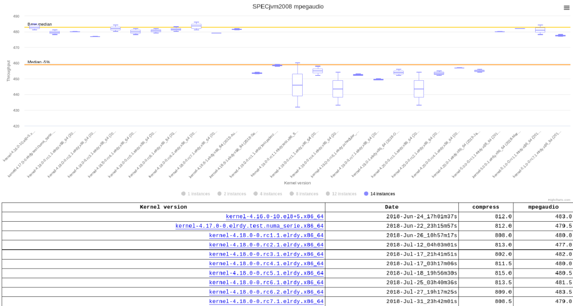
Figure 5.3: Generated box plot timeline graph of mpegaudio operation from SPECjvm2008 benchmark with part of table showing numeric results of the SPECjvm2008 operations. The table shows medians from benchmark runs with featured number of threads and the kernel names are links to our team database of results. It displays performance results of upstream kernels for Red Hat Enterprise Linux 8. The performance degradation is consequence of changes in memory placement and migration behavior.
