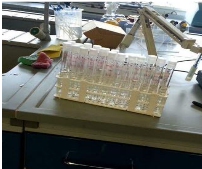
Fig. 9 Pore collection with rhizon samplers or/suction cups ready for analysis .
