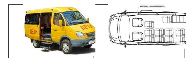
Color of a body – yellow. The speed limiter to 60 km/h Lamp of external lighting over a movable door The ventilating hatch in forward part of salon Footboard side with an additional step The device interfering a bus start of motion at an open door Hand-rail in passes
