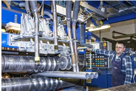
Fig. 10 SAW welding of membrane walls. [11]
