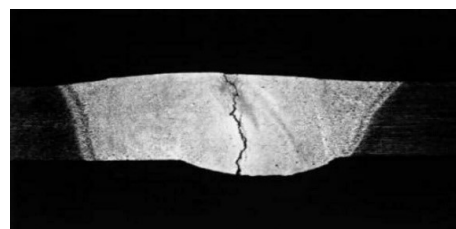
Fig. 24 Cut of solidification crack [41]
