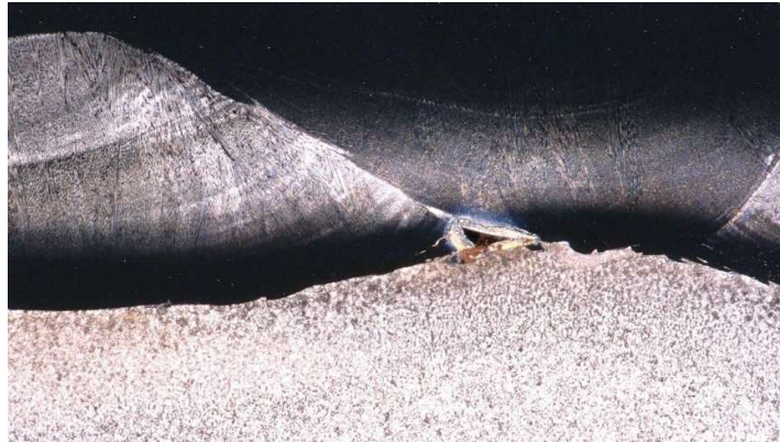
Fig. 47 Detail of crack in specimen I
