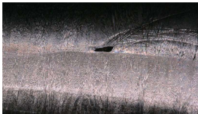
Fig. 51 Detail of crack between the layers 100x
