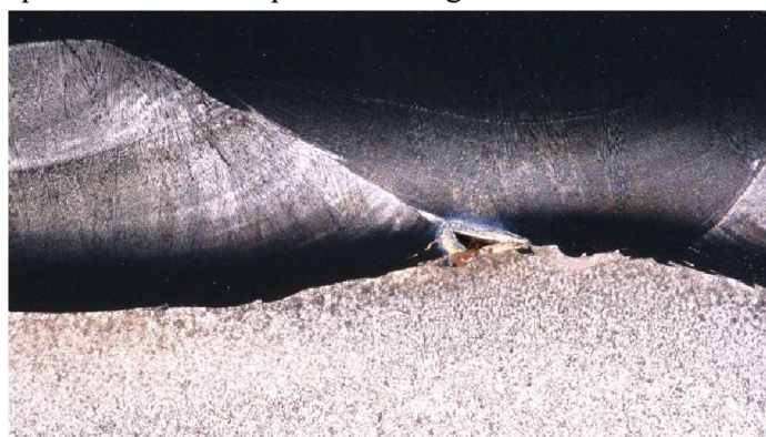
Fig. 47 Detail of crack in specimen I
