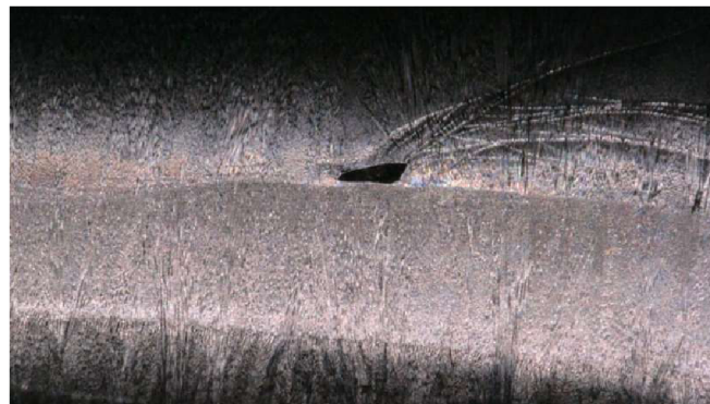
Fig. 51 Detail of crack between the layers 100x
