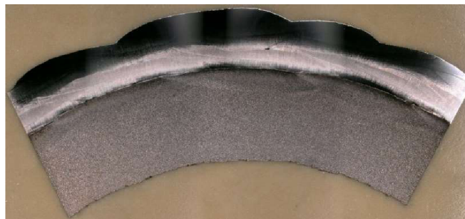
Fig. 50 Panorama of sample with Inconel 625 structure
