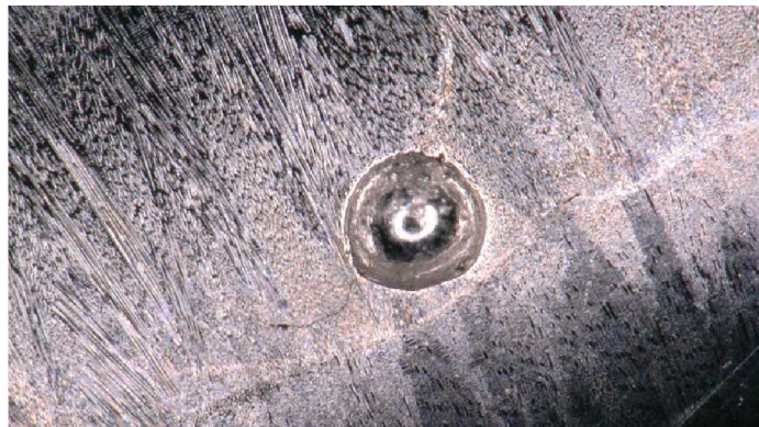
Fig. 53 Detail of the bubble in overlay
