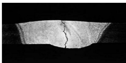
Fig. 24 Cut of solidification crack [41]
