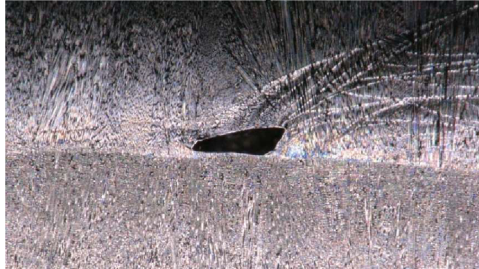
Fig. 52 Detail of crack between layers
