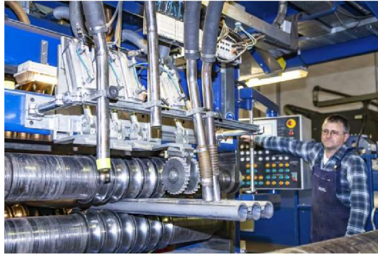
Fig. 10 SAW welding of membrane walls. [11]
