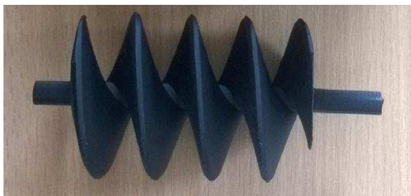
Figure 23. 3D printed auger drill (Archimedes screw)
