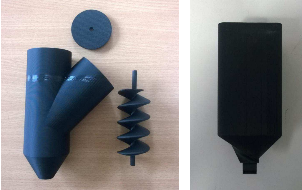
Figure 26. Printed prototypes of the first and second designs
