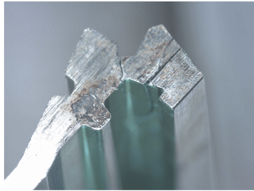
Figure 2.5: Fatigue cracks on core 532
