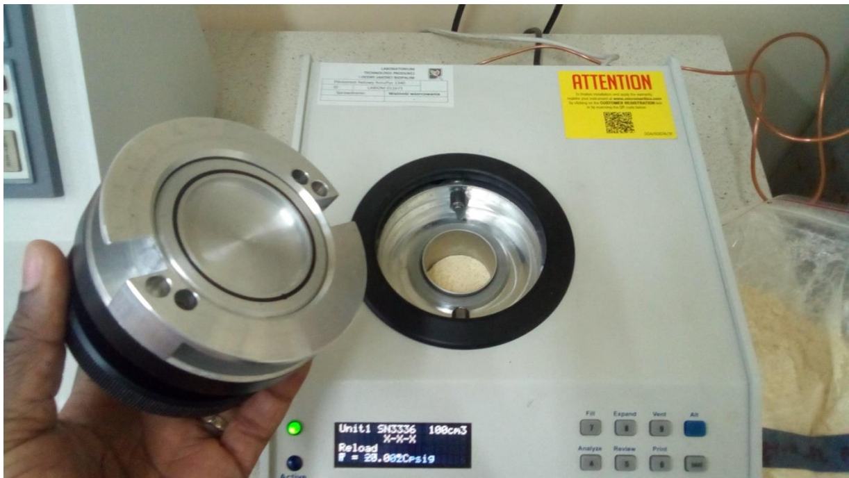
Plate 4.2. True density measurement system
