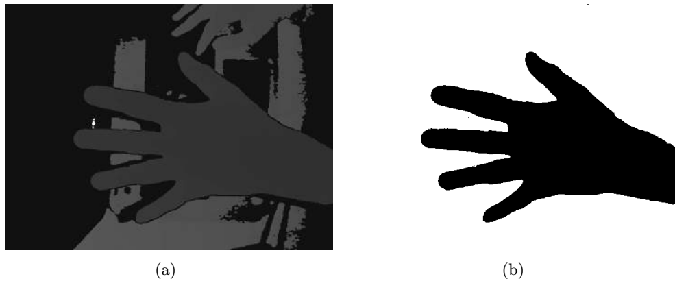
Figure 3.5: Foreground - background separation using the depth information: (a) Input depth map; (b) Output hand mask.
