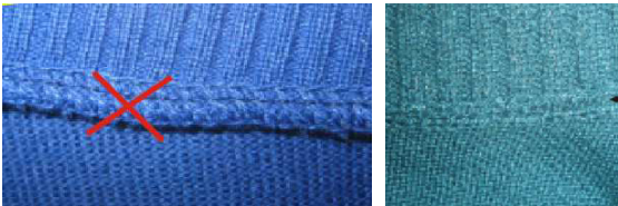
Looping assembly for neckline band.
