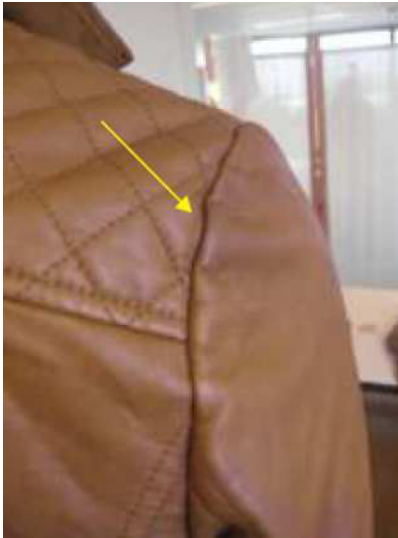
Excess fabric at head of sleeve NOT OK
