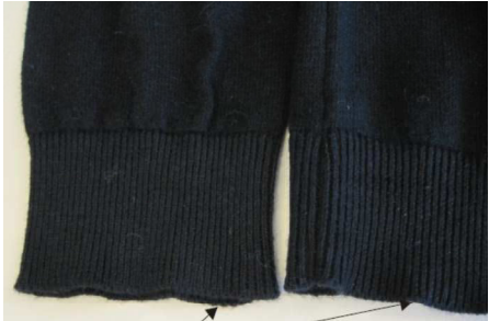
LFA more tighten / bottom is loosen NOT OK
