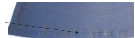
Bottom hem stretched out NOT ACCEPTABLE
