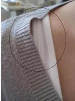
NOT OK / ribbing loosen
