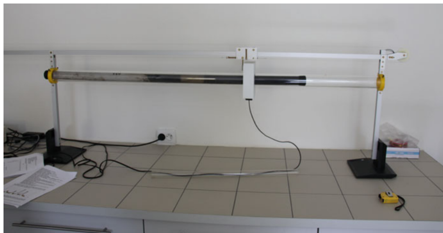
Fig. 33.4 Magnetic susceptibility measurement on the boreholes drilled on Spolchemie Site I
