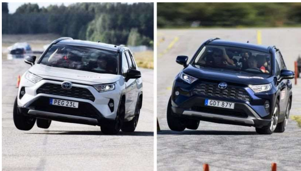
Obr. 54 Losí test automobilu Toyota RAV4 [44]
