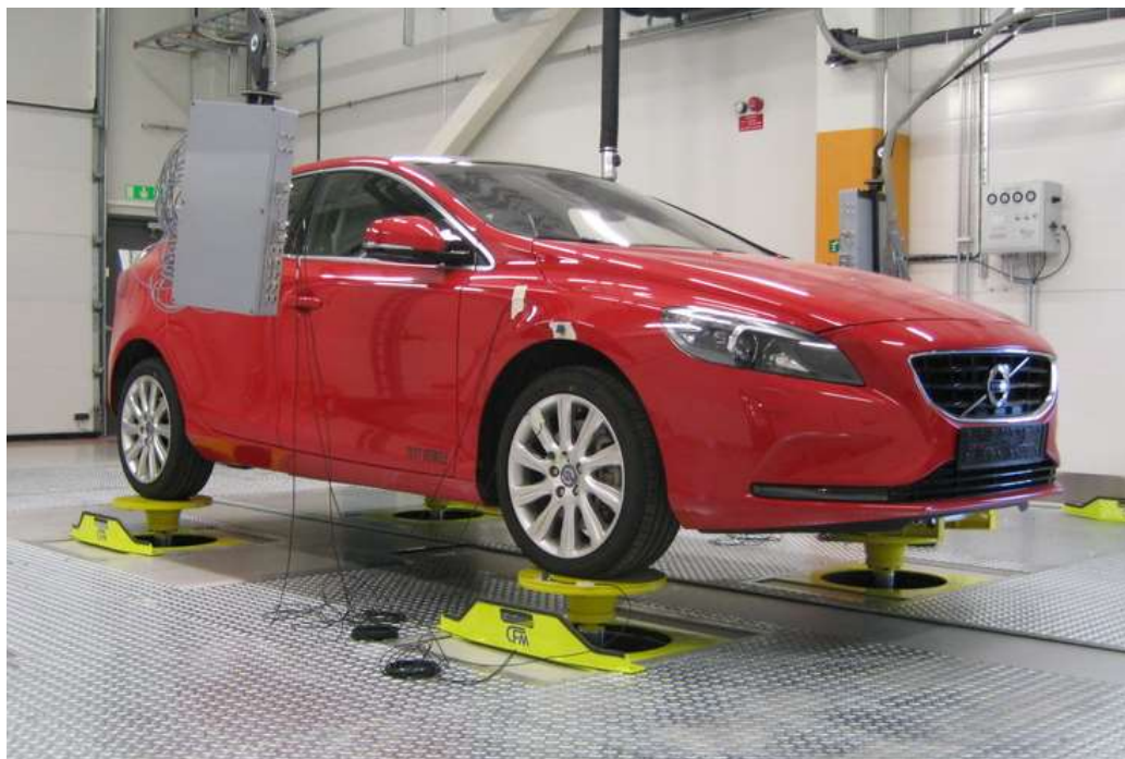
Obr. 26 Four-post test rig [31]
