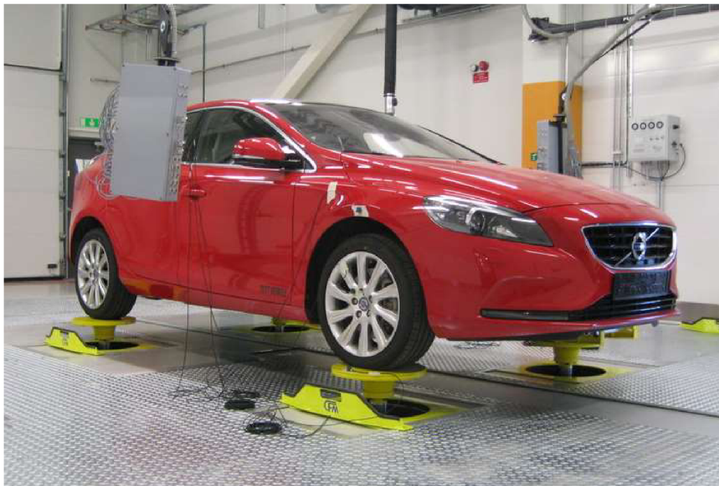
Obr. 26 Four-post test rig [31]
