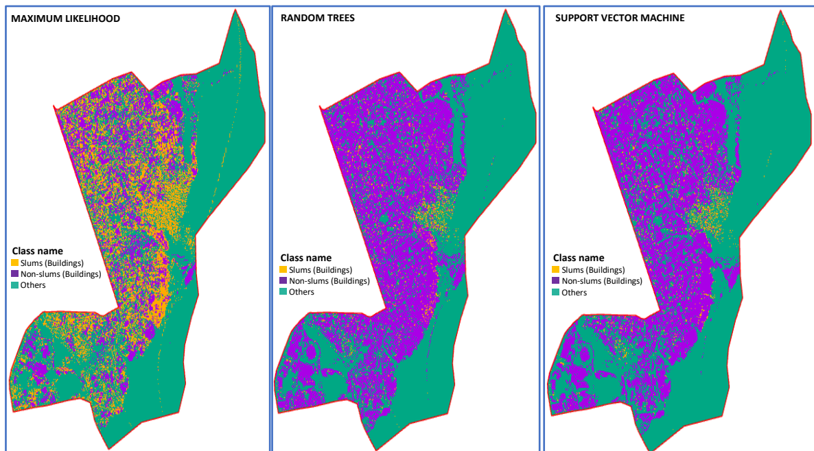
Fig 38 Pixel-based classification result from Sentinel-2 imagery of Lagos Mainland
