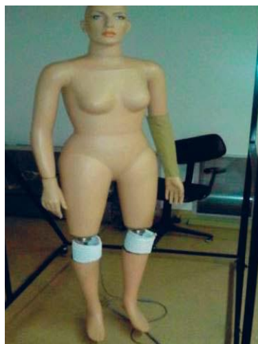
Figure 4: Thermal manikin Maria with left forearm covered with sample of firefighter protective clothing
