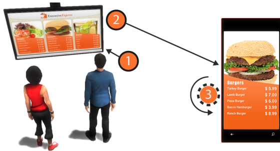
Figure 5.1: The PeepList interaction overview. 1) User approaches pervasive display that is equipped with an eye-tracking technology. 2) While user examines the content of the pervasive display, the PeepList system (a part of the pervasive display) internally reorders relevance for on-screen elements based on user's eye tracking data. Reordered items are automatically sent to user's mobile device. 3) After the interaction, the user has access to personalized results and is able to further filter and reorder the results.
