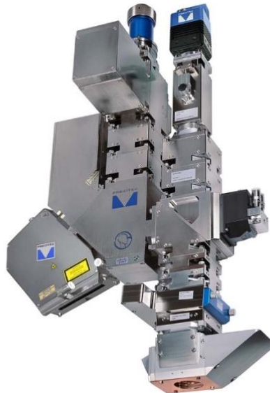
Obr. 23 Laserová hlavice WeldMaster 4.0 Scan&Track and Inspect [28]
