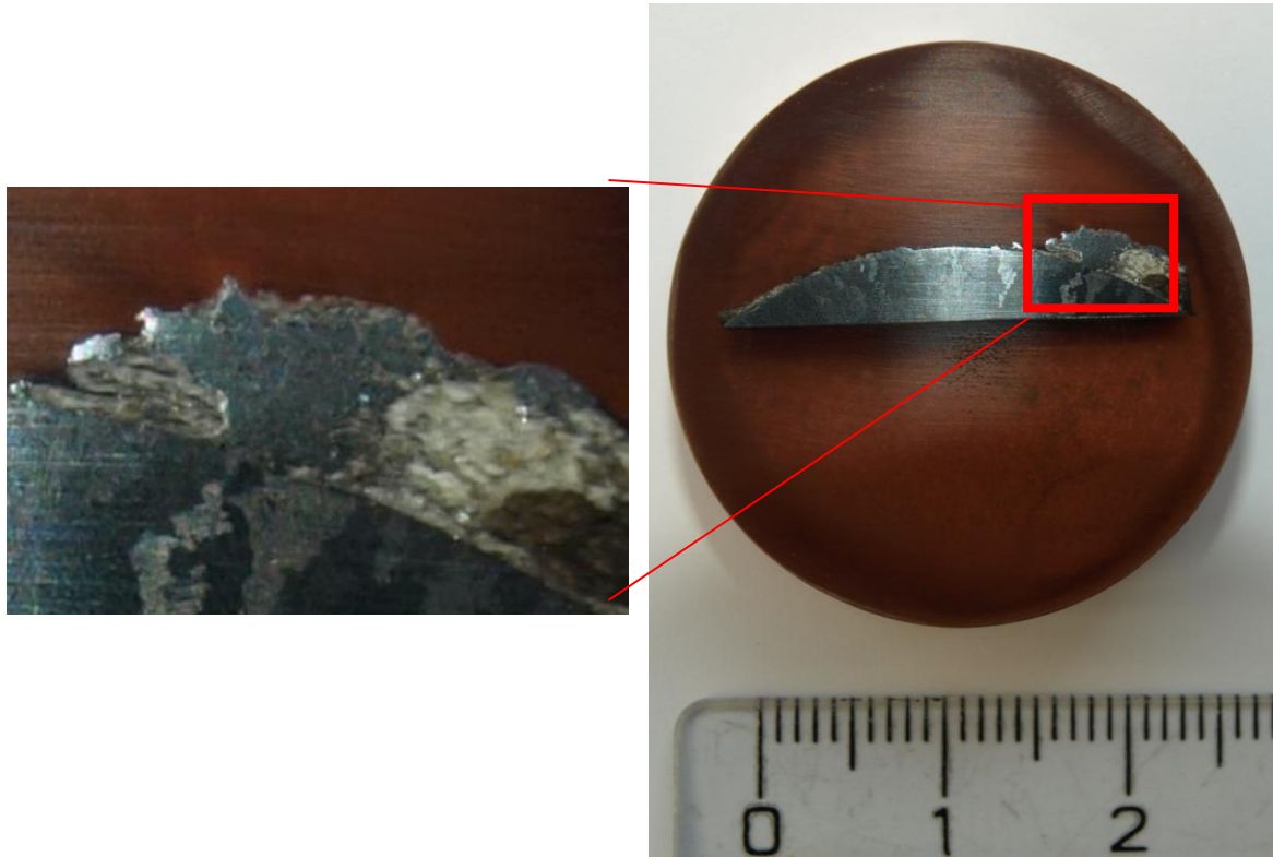
Fig. 42: Overview of the small piece of the TiAlNb alloy with a part of the crucible wall attached after melting and re-solidification. The area marked by a red rectangle indicates a position where the melt penetrated into the crack in the crucible wall.
