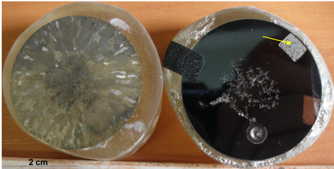
Fig. 21: Overview image of metallographic cross-sections, samples of the melt T3.
