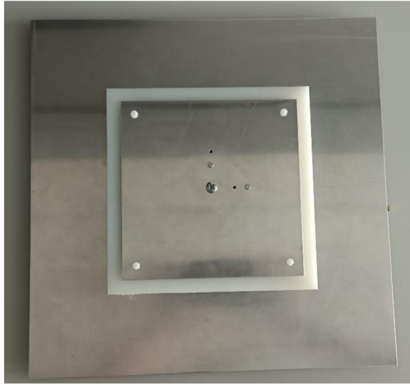
Fig. 5.3: The fully build single antenna (top view)
