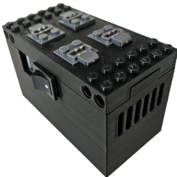
Figure 7.5: 3D printed enclosure for the second driver iteration
