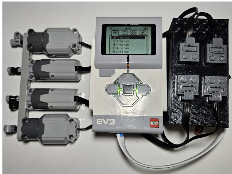
Figure D.3: Driver V0.2 connected to the EV3 and four Power Functions motors
