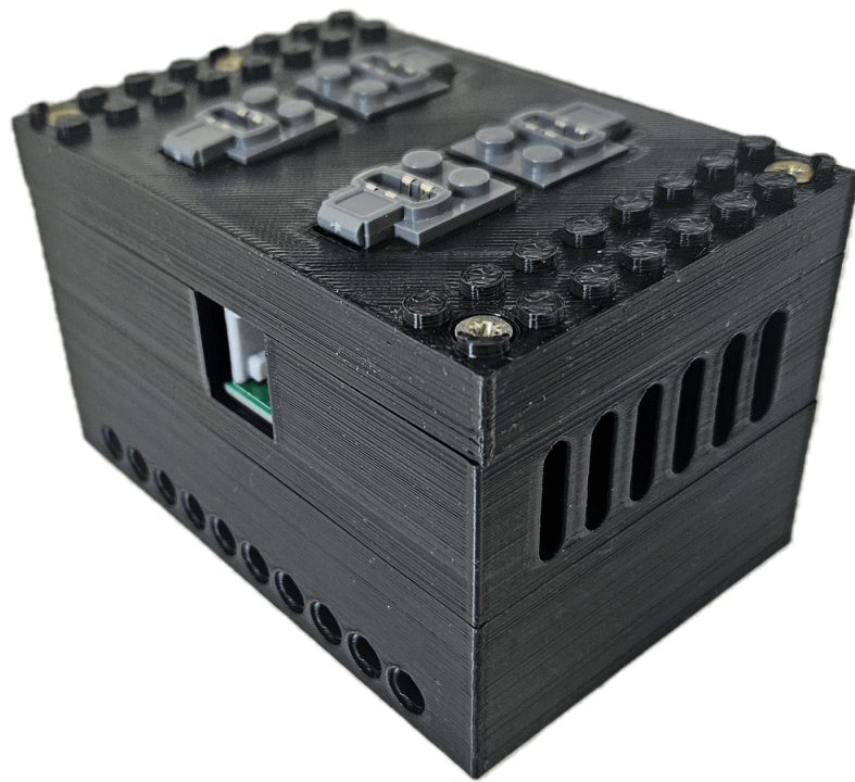
Figure 6.9: 3D printed enclosure for the motor driver
