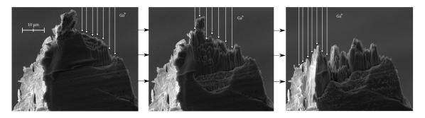
Figure 4.15: Three pictures show SEM view after three steps of GaN beam scattering of Pt/Ir. For original view refer to figure 4.11
