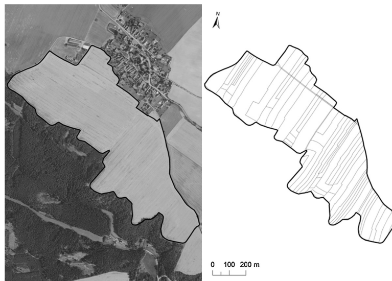
Fig. 1. An example of land-ownership fragmentation, using samples from the study. Left: a production block of 52.6 ha, traced over an orthophotograph (Source: LPIS). Right: ownership pattern – 82 parcels with an average size of 0.64 ha. (Source: Czech Office for Surveying, Mapping and Cadastre).
