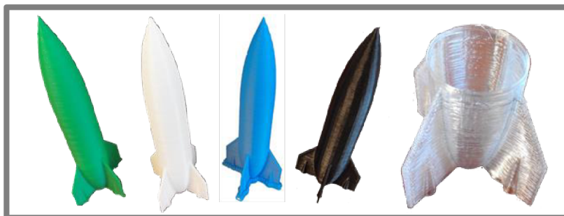
Obr. 4-28 Zleva PLA-D, PC, PLA, ABS, a PET
