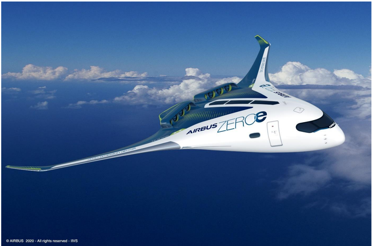
Obr. 6.2 Koncept blended wing body [52].
