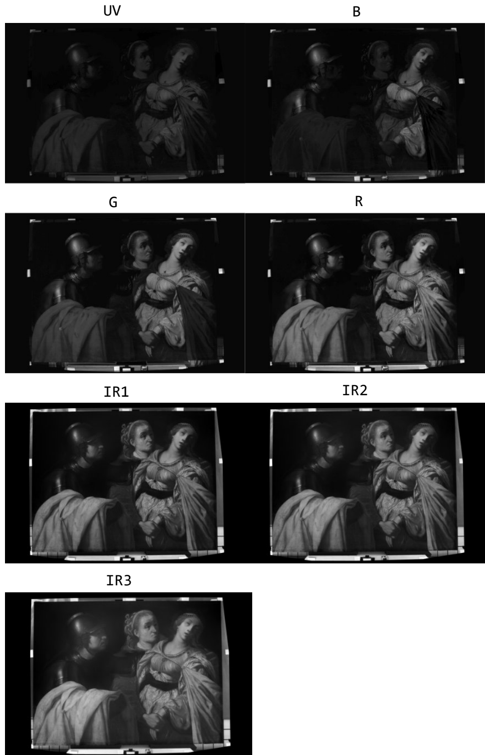
Figure 4.10: Result of Software extrapolated multispectral imaging mode processing - multispectral images in the range from UV to IR.
