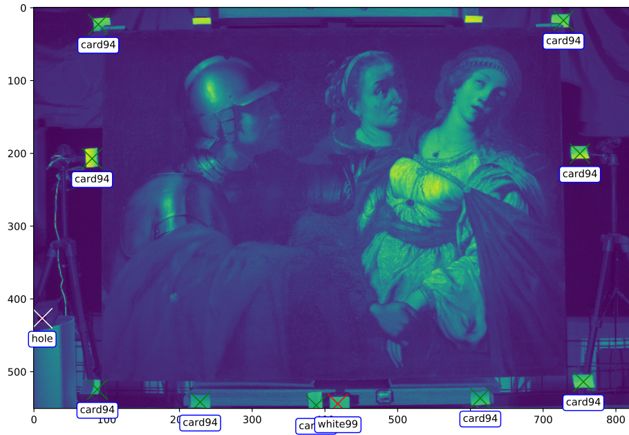
Figure 4.5: Marking the black hole, the white standard and the white cards.
