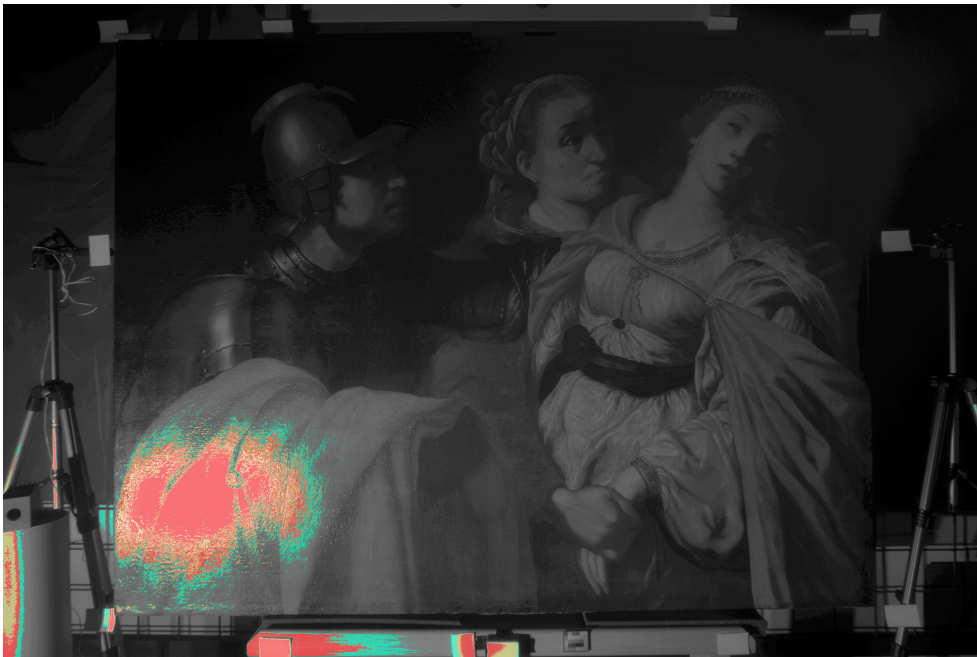
Figure 4.3: Exposure checking. Red color stands for overexposed pixels.
