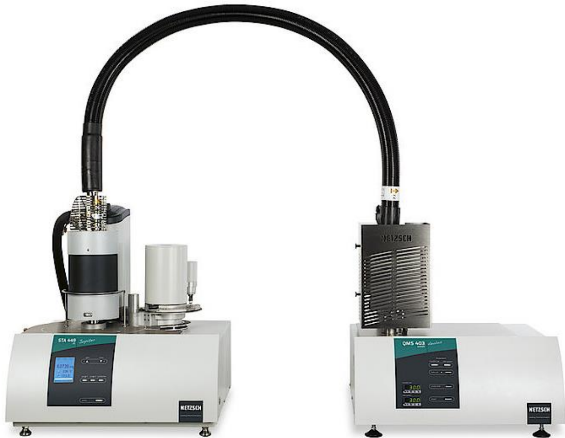
Figure 9.1 Coupling TGA-MS via capillary; TGA analyser STA 449 F3 Jupiter and mass spectrometer QMS 403 C Aëolos (NETZSCH, Germany) [73].
