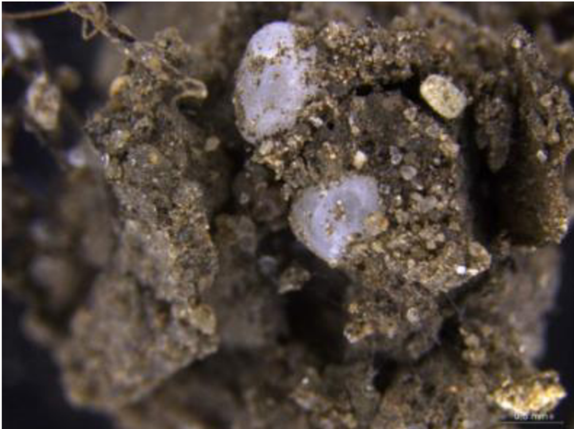
Figure 2.3 Microplastic items (polyethylene of 1.18–1.4 mm size) incorporated into soil via earthworm transport [34].
