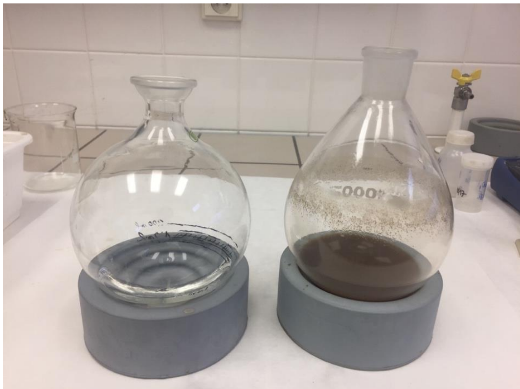
Figure 15. Thickened LPD (right) and distillate (left) obtained from the vacuum evaporation of 200 mL nitrified LPD. Source: Author.
