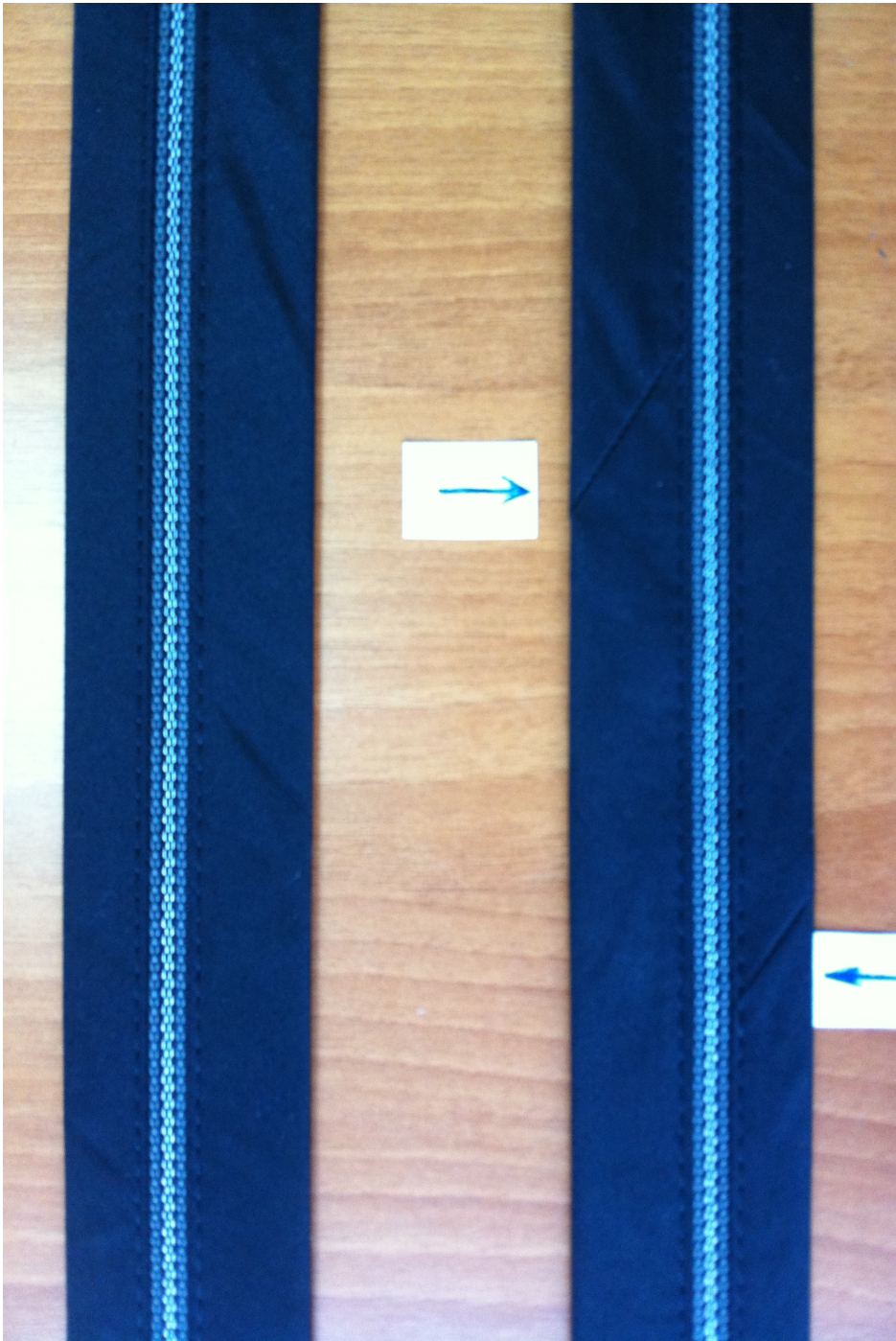
Picture 11 Example of butt joint defect on waist band
