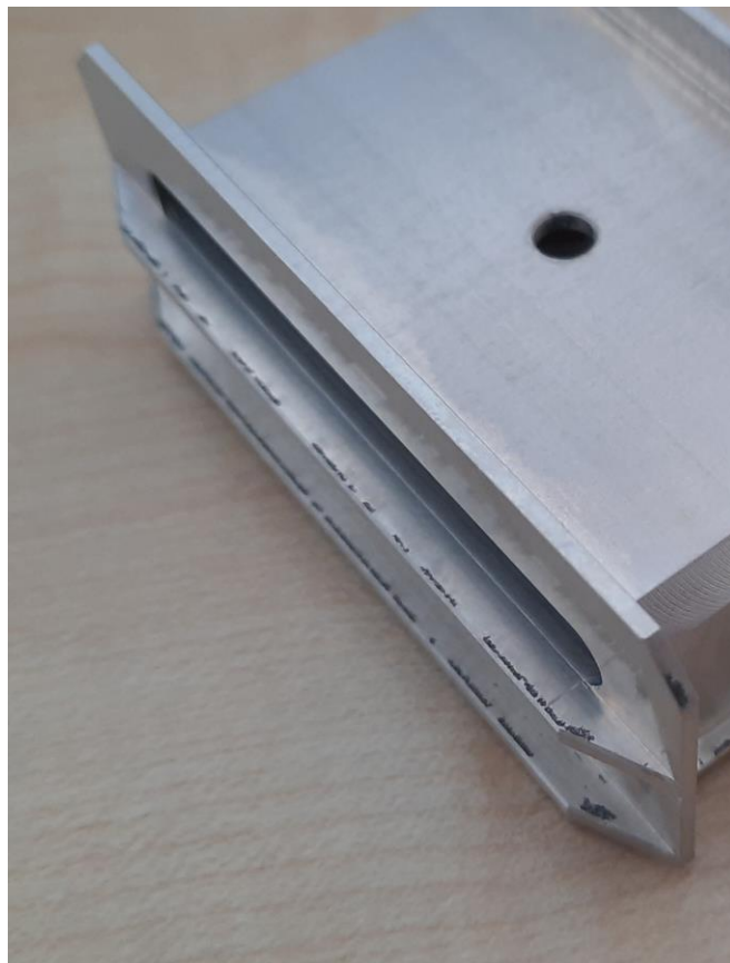
Figure 10.31: Defects of the ribs, left side.
