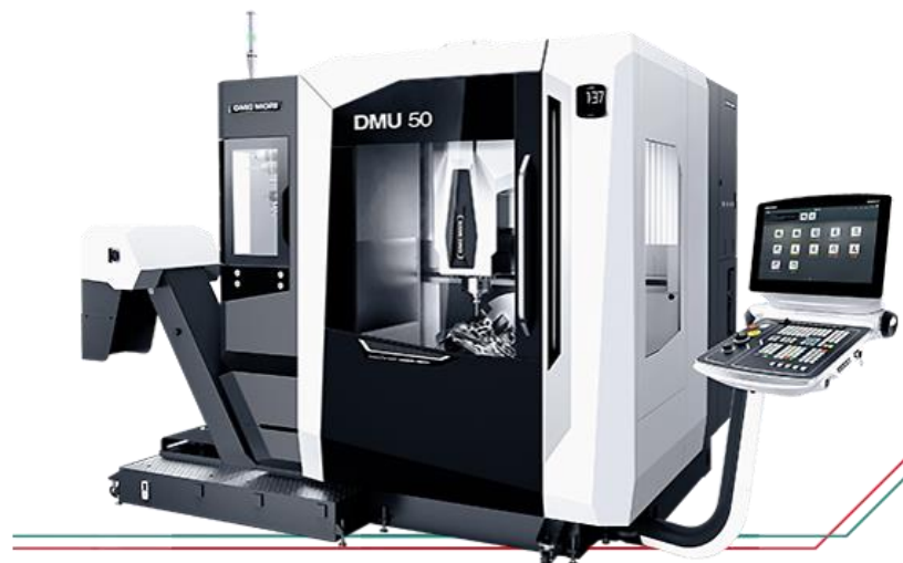
Figure 10.1: DMG Mori DMU 50 3 rd generation [35].
