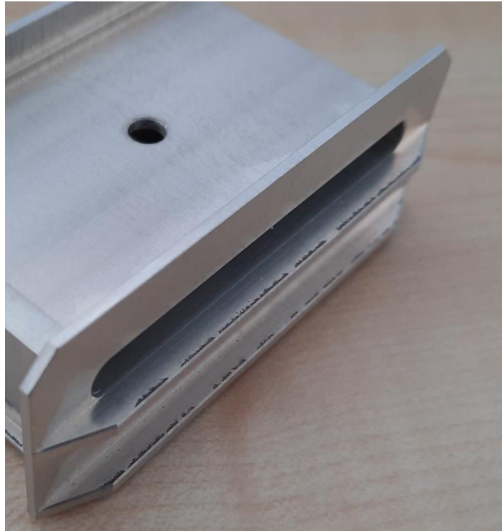
Figure 10.30: Defets on the ribs, right side.
