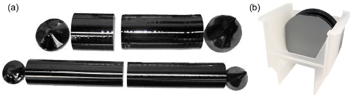
Figure 3.5: (a) Silicon single crystal cut into pieces. (b) Polished silicon wafers in the cassette.
