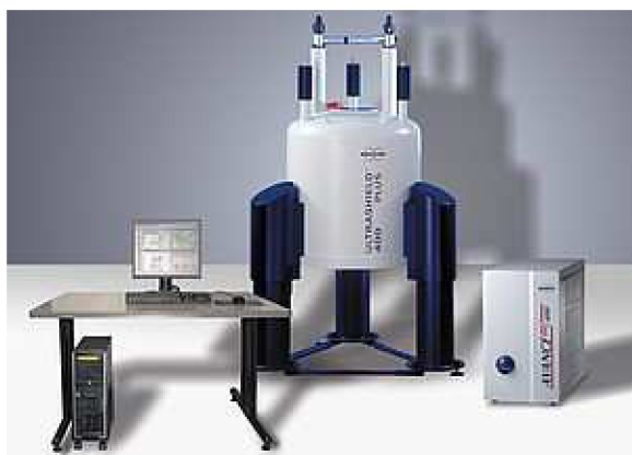
Fig.22 NMR spectrometer Bruker Avance III 500 MHz
