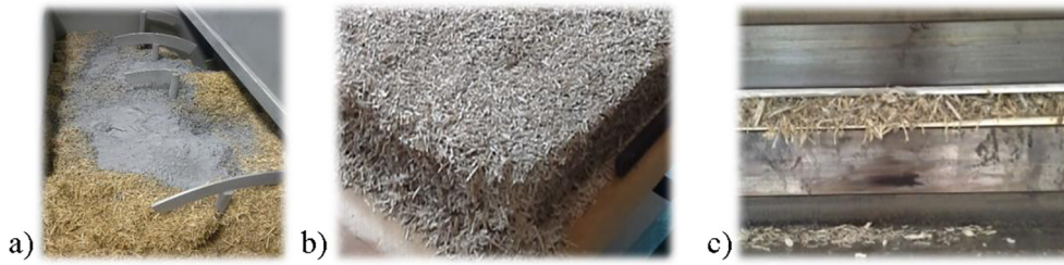
Fig. 2. The production of our developed materials: a) mixing adhesive with modified particles, b) layering particles, c) pressing in laboratory press.
