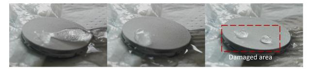
**Figure 35** Degradation of water-mobility performance of the A3-D YSZ modified sample after water-flush test
