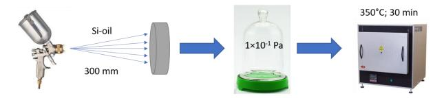
Figure 20 Illustration of silicone oil surface treatment
