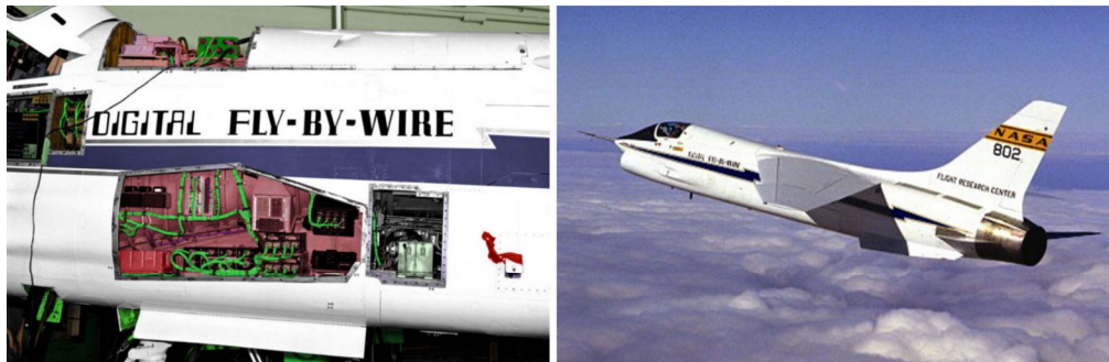
Figure 1.3: Vought F-8C Crusader equipped with a digital FBW system. Sources [65, 66]
