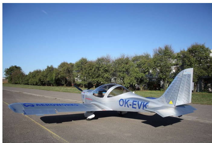
Figure E.9: Experimental LSA with control surface operated by EMAs.
