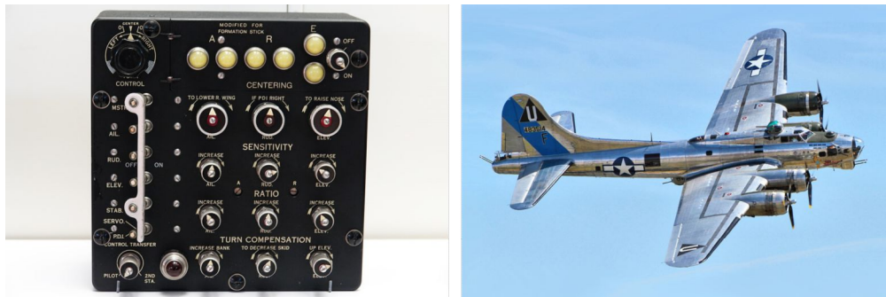
Figure 1.2: Honeywell C-1 autopilot control panel. Sources [1, 3]
